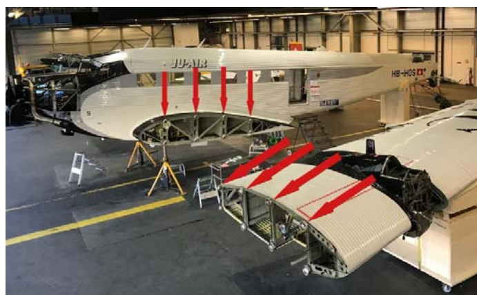
Figure 7 Disassembled Ju-52 wing showing the connection points
