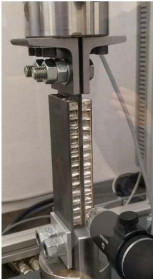
Fatigue test of sandwich sample under shear loading. Core cells continually checked for cracking, yet no cracks detected near partially filled core cells
