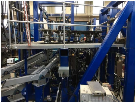
Figure 31 Test Configuration of FTS2 Fatigue Test
