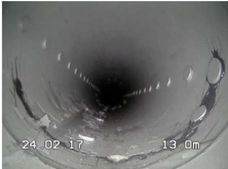
Figure 11 Borescope inspections of the cracked spar II
