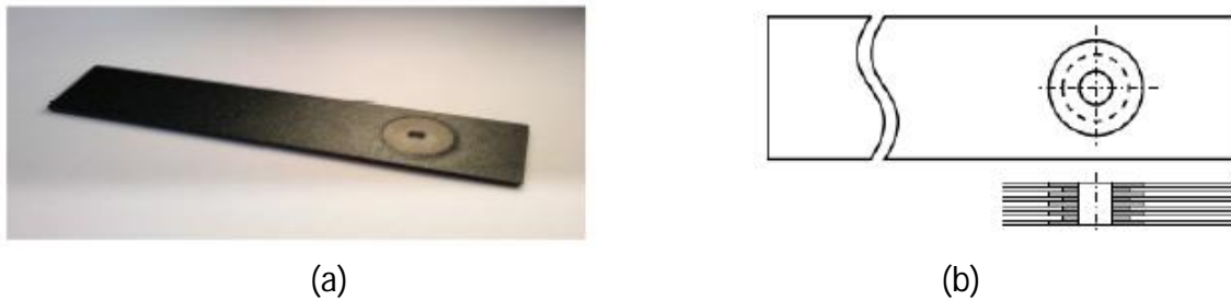
Figure 3.2-1. A specimen with a patched metal insert (a) and a schematic of the insert geometry (b).
