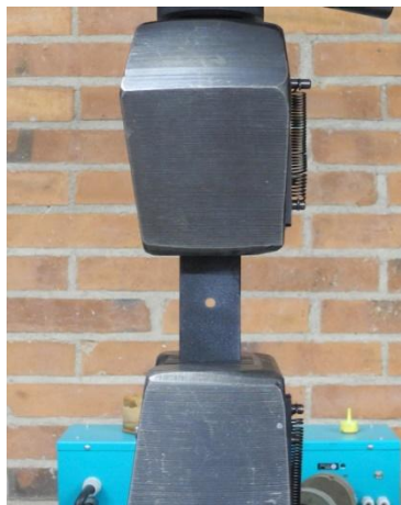
Figure 3.2-9. Test setup for open-hole tensile tests.
