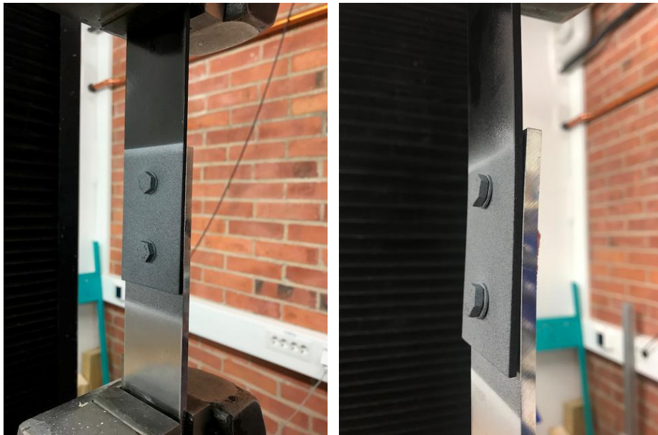
Figure 3.2-13. Test setup for single-shear test.
