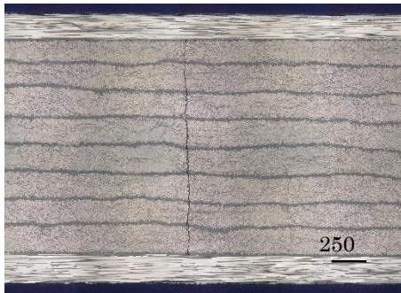
Figure 3.2-1. Transverse crack observed on the specimen edge surface. ( \epsilon_{\max} = 0.15\% , N = 4.3 \times 10^8 cycles)
