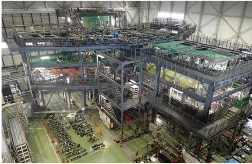
Figure 5.1-1. MRJ90 full scale fatigue test setup
