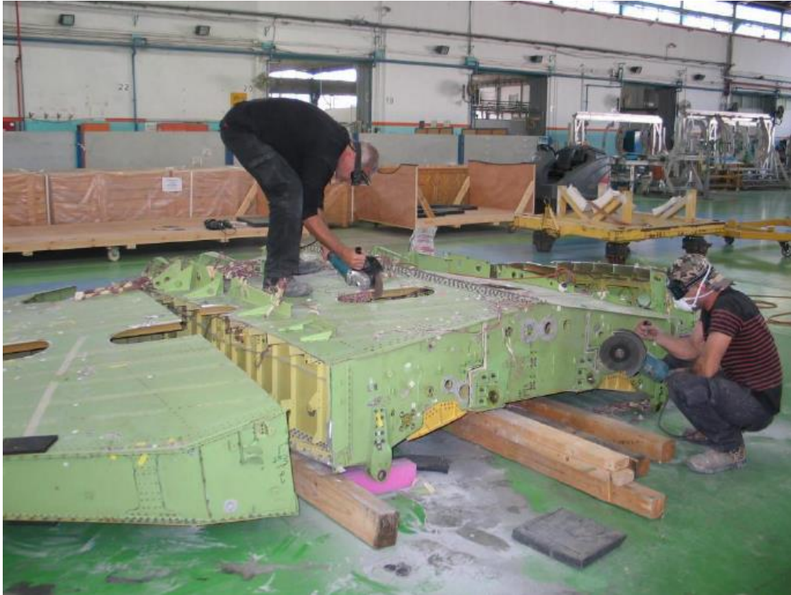
Figure 1. Preparation for teardown inspection
