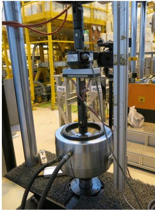
Figure 12. The tested specimen at the loading fixture
