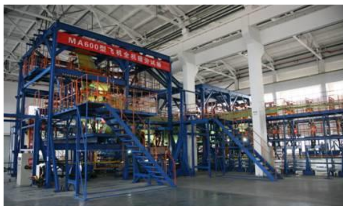
Figure 5-6 MA600 full-scale fatigue test
