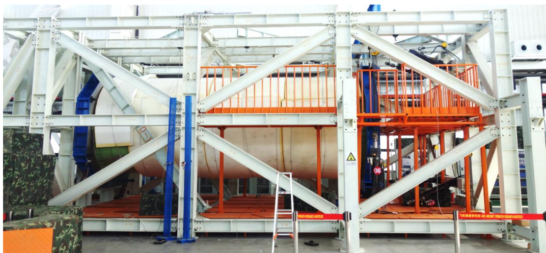
Figure 6-8 Self-balancing overall support loading framework
