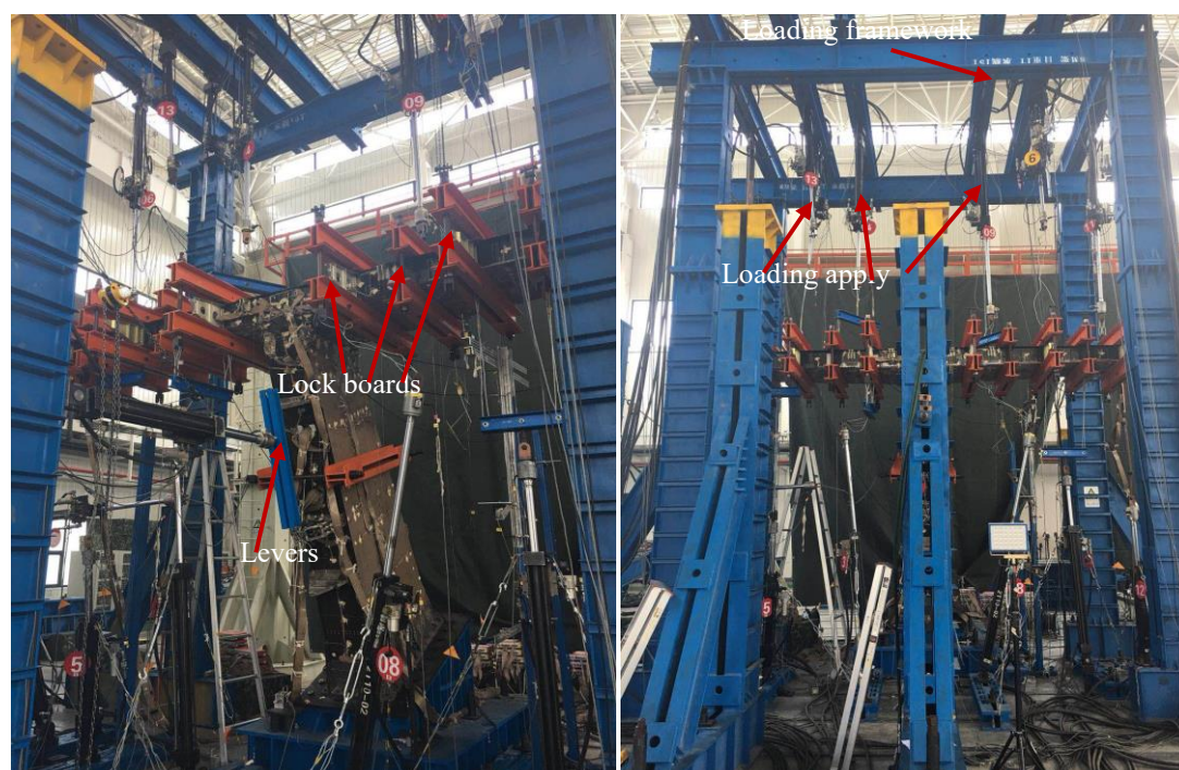
Figure 6-15 Local load test of horizontal and vertical tails
