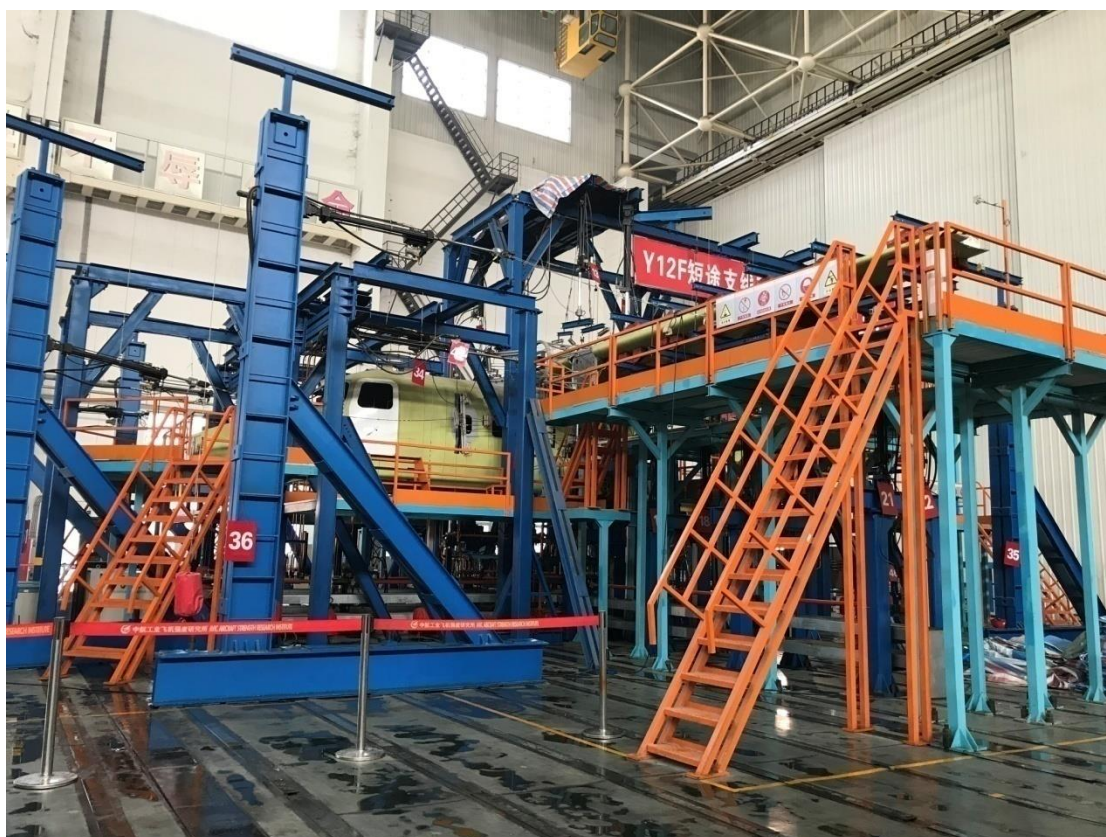
Figure 6-17 Full-Scale Fatigue Test of general aviation aircraft
