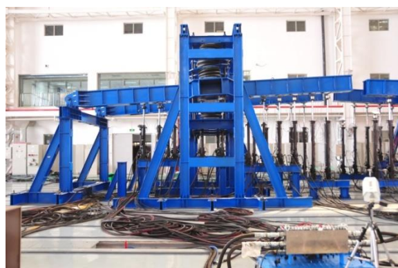
Figure 5-29 Wing adjusting-stiffness test bench(WASTB)
