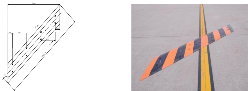
Figure 6-24 The shimmy board of landing gear shimmy test for ARJ21 aircraft
