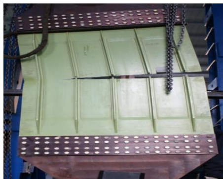
Figure 3-22 Damage tolerance test of integral wing lower panel
