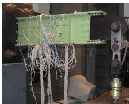
Figure 3-23 Fatigue and damage tolerance test of integral wing spar
