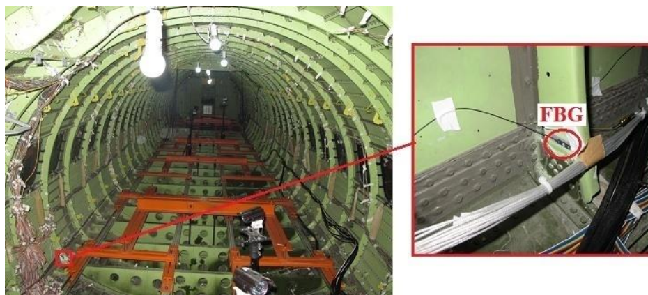
Figure 6-1 Strain monitoring of fuselage using FBG
