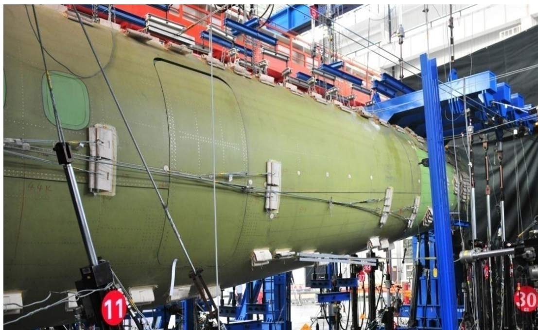
Figure 6-11 The Mid-rear fuselage stiffness and strength test
