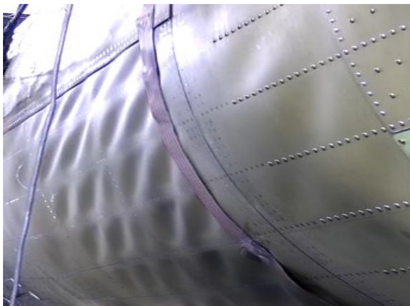
Figure 6-13 Fuselage skin buckling tension field
